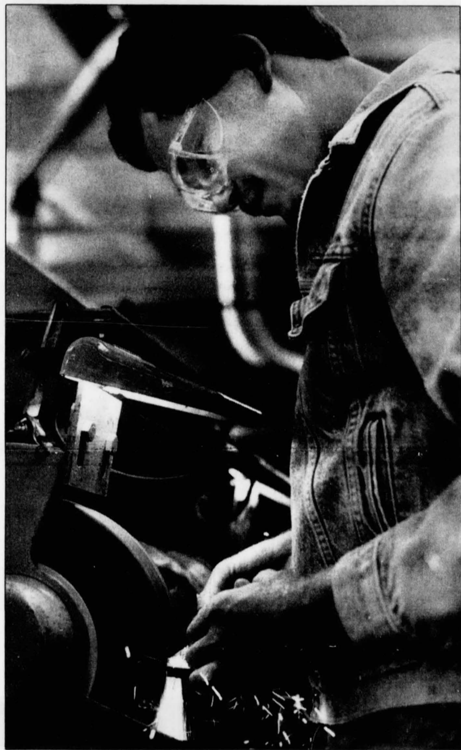
A flector test? That's what electrical computer technology junior Tom Brounger is doing. He welds two pieces of metal together and then breaks them apart to test the strength of the fusion.
